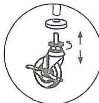
4. Carefully place the trolley on the ground and ensure all the castors are touching the floor. Turn the screws tightly with the Allen key. Use the wrench included to turn the nuts tightly.
