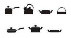
Due to the particular nature of the induction field, the cookware must have a plane magnetic bottom (a magnet must stick to it).
